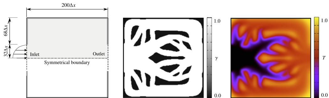
Figure 2.22: Heat exchange maximization problem: design domain and boundary conditions (left), optimized configuration (middle), normalized temperature distribution (right), taken from [102].
