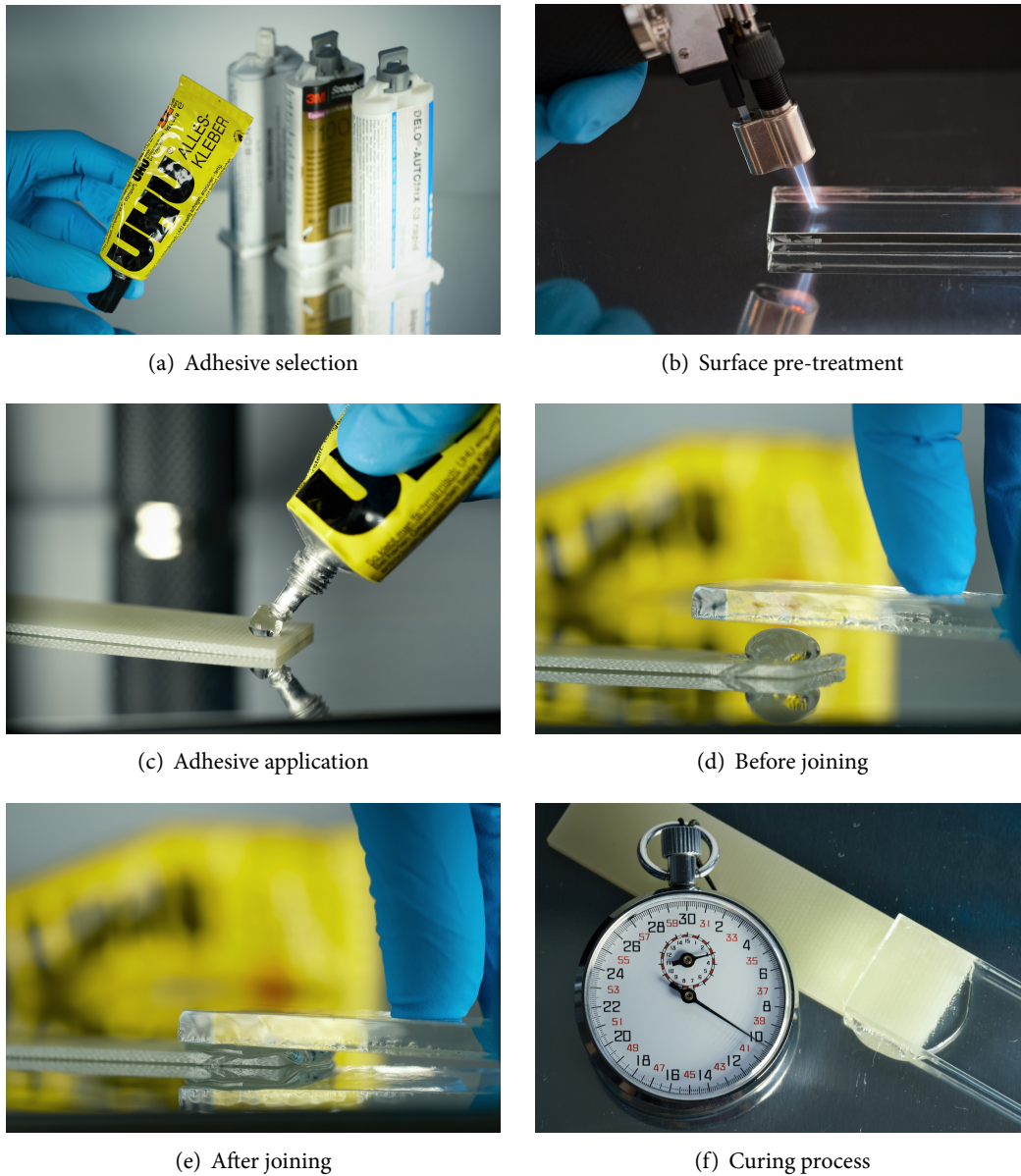
Figure 2.1: Manufacturing process of adhesively bonded joints.
